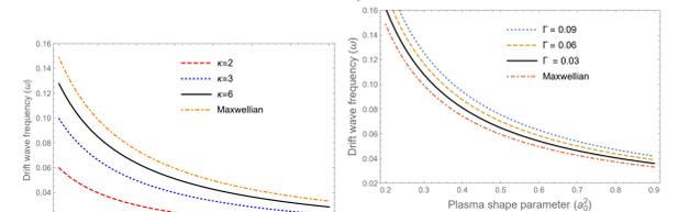
(c) Variation of frequencies of the drift waves in a D-T for different values of  $\Gamma$  (for plasma for different values of Cairns distributed electron)  $\kappa$  against plasma shape parameter  $a_0^2$ . (d) The frequencies of the drift waves for D-T plasma against plasma shape parameter.
