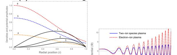
(a) Radial potential profiles presenting the amplitude  $\Phi(r)$  in curves 1-3. The curves 4, 5 and 6 show, (b) The potential profile for respectively the equilibrium (a) single ion plasma red density profiles of ions  $a, b$  dashed curve and (b) two-ion species solid blue curve.
